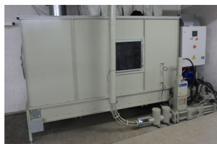
FVB250 FDK push floor with two screw conveyors, can be retrofitted with a second briquetter
